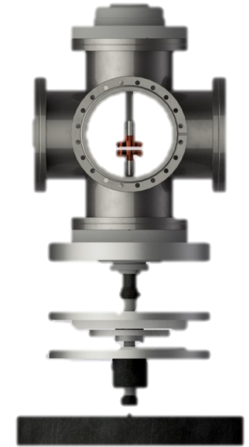
Model vacuum interrupter with Thomson coil actuator
